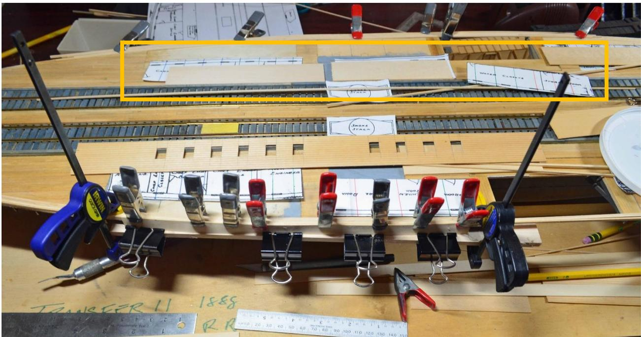
No. 4: 4 The open windows completed. The sidewalls will be cut to length.
